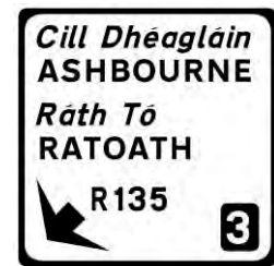
Figure 2.5.17: Typical Regional Route Exit Taper Gantry Sign
