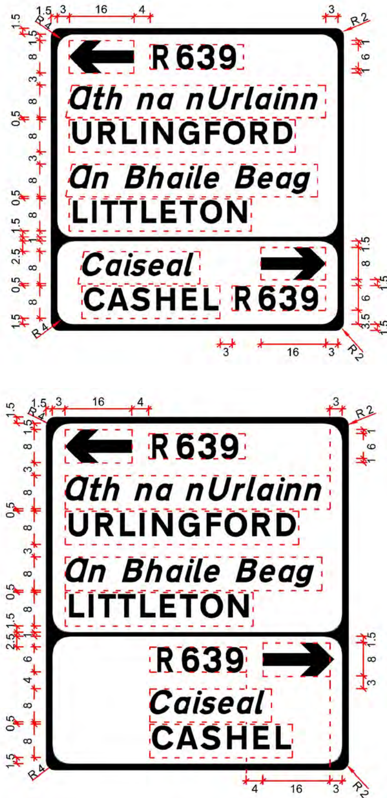
Figure 2.6.13: Stack Sign with Multiple Destinations in a Panel
