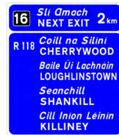
Figure 2.4.6: Typical 2km Next Exit Sign
