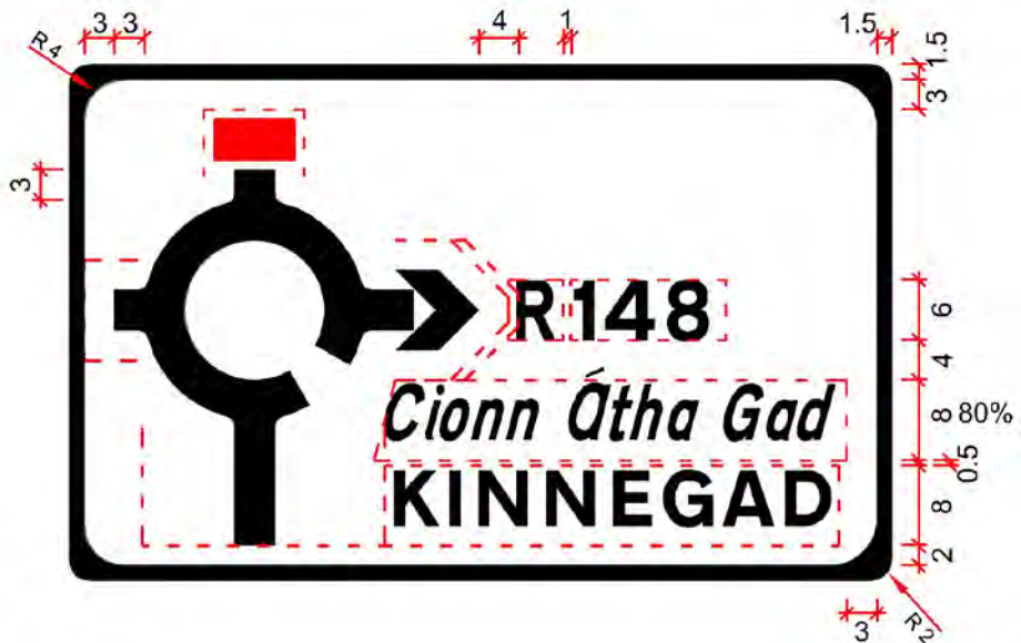
Figure 2.6.33: Map Type Roundabout Sign on Regional Route with Stub and 'No Entry' Arms
