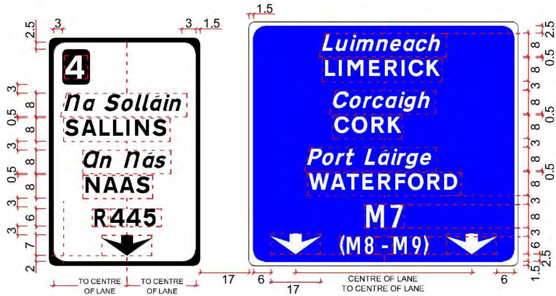
Figure 2.4.26: Lane Drop Gantry Sign at the Start of a Motorway and Reduced Height Diverge Panel
