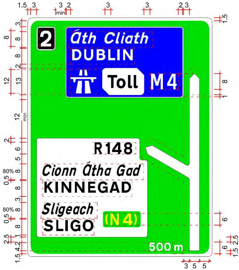
Figure 2.5.26: 500m Advance Direction Sign to Start of Motorway
