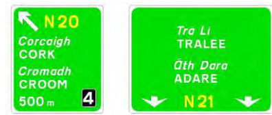
Figure 2.5.8: Typical Non-Lane Drop Gantry at 500m.
