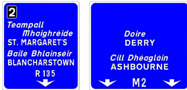
Figure 2.4.23: Typical Lane Drop Gantry Sign
