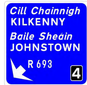
Figure 2.4.27: Typical Exit Taper Gantry
