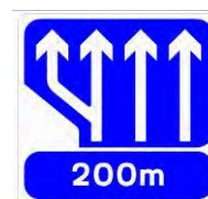
Figure 2.4.2: Typical Lane Gain Signs
