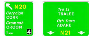
Figure 2.5.9: Typical Non-Lane Drop Gantry at 1km.
