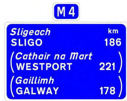
Figure 2.4.49: Typical Route Confirmatory Sign.
