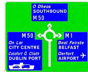
Figures 2.6.23: Map Type Sign for Start of Motorway with Motorway Legend Panels
