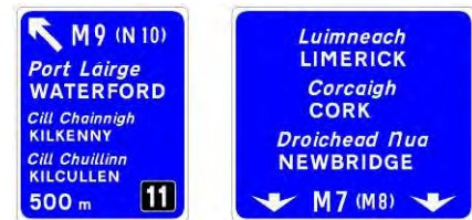
Figure 2.4.11: Typical Non-Lane Drop Gantry
