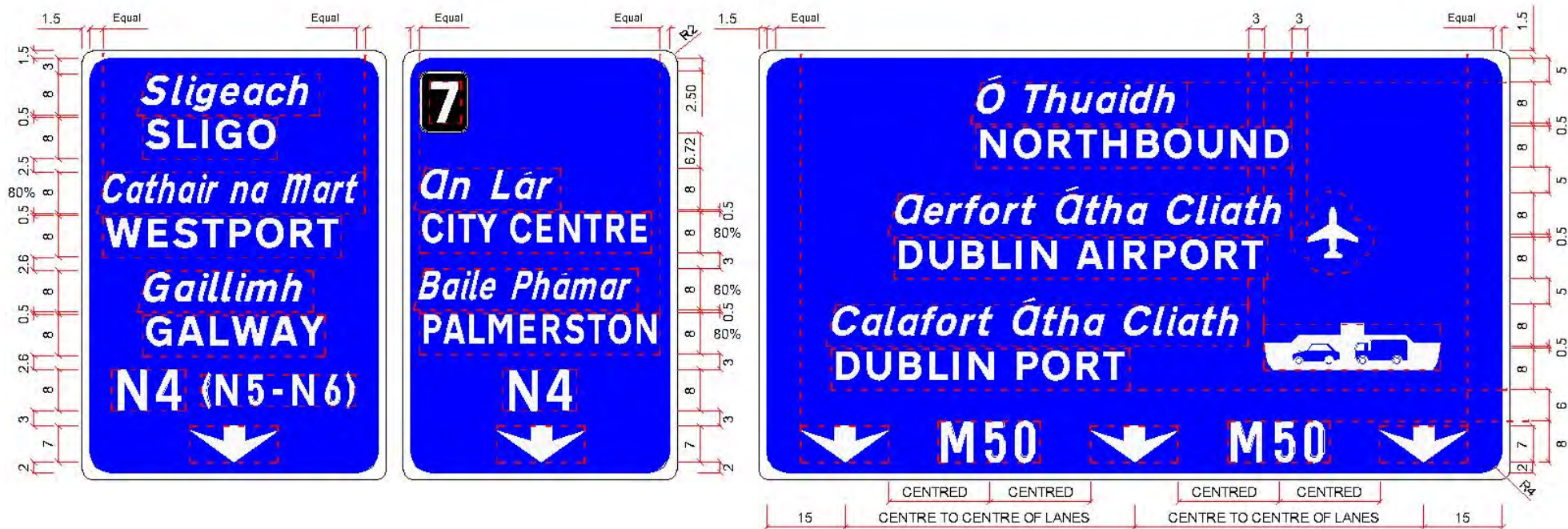
Figure 2.4.25: Lane Drop Gantry Sign at a 2-Lane Diverge
