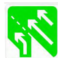
Figure 2.5.2: Typical Lane Gain Sign
