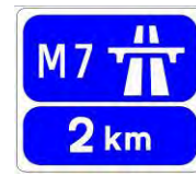
Figure 2.5.3: Sign F 332: Motorway Regulations Ahead
