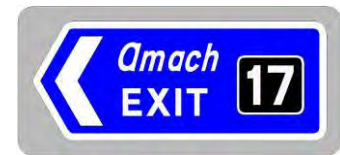
Figure 2.4.42: Typical Exit Sign
