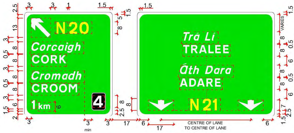
Figure 2.5.12: 1km Non-Lane Drop Gantry Sign with Diverge to a National Route
