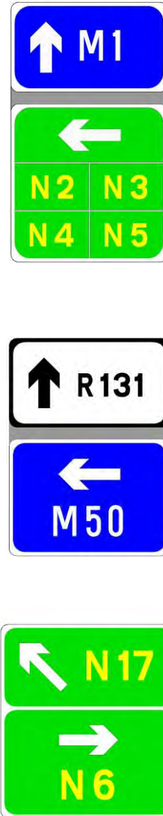
Figure 2.6.16: Typical Examples of Route Direction Signs
