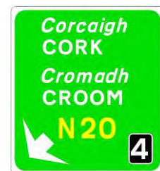
Figure 2.5.18: Typical National Route Exit Taper Gantry Sign
