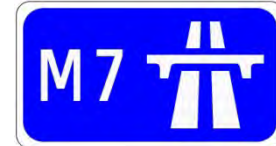
Figure 2.4.3: Sign F 330: Typical Start of Motorway'
