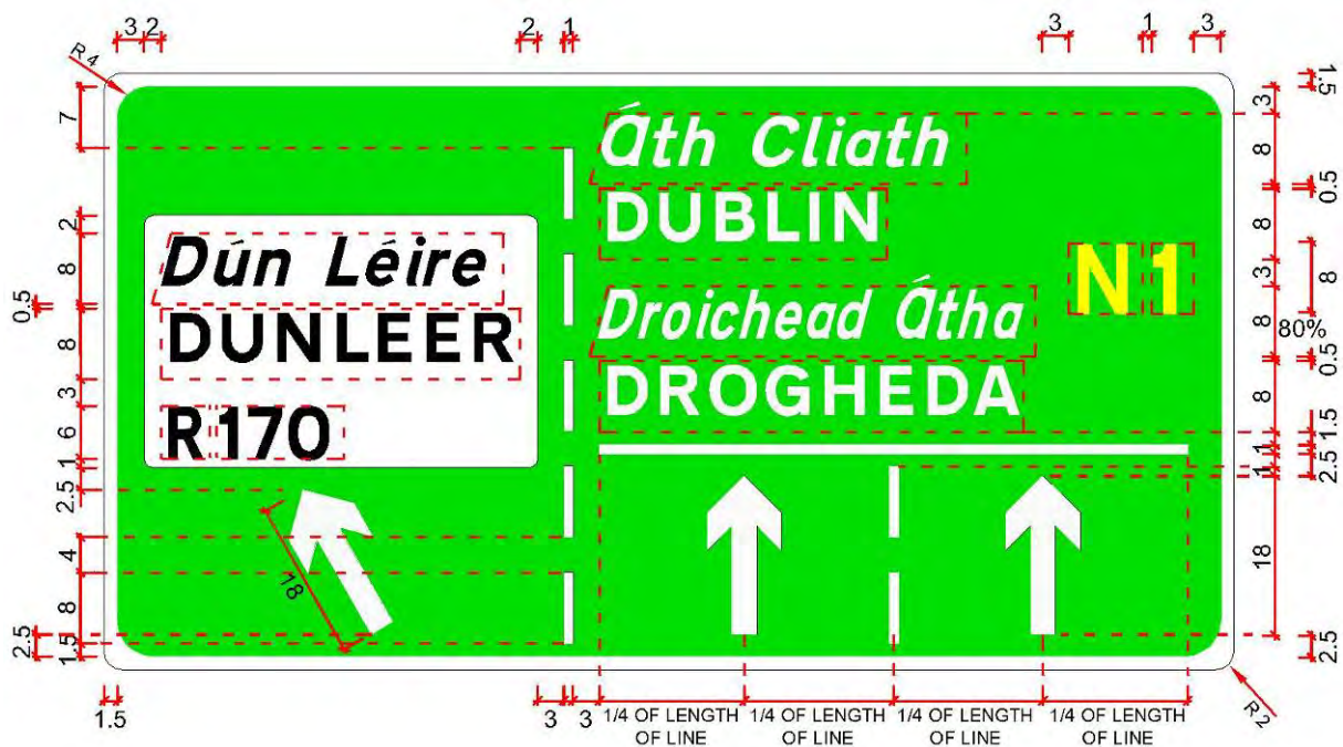
Figure 2.6.51: Lane Destination Sign in Advance of a Regional Route Exit
