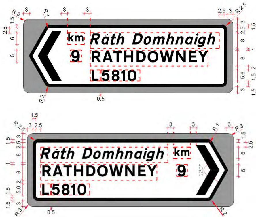
Figure 2.6.71: Layout of Direction Signs with a Distance (Pointing to the Left and Right)
