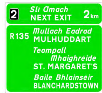
Figure 2.5.5: Typical 2km Next Exit Sign.
