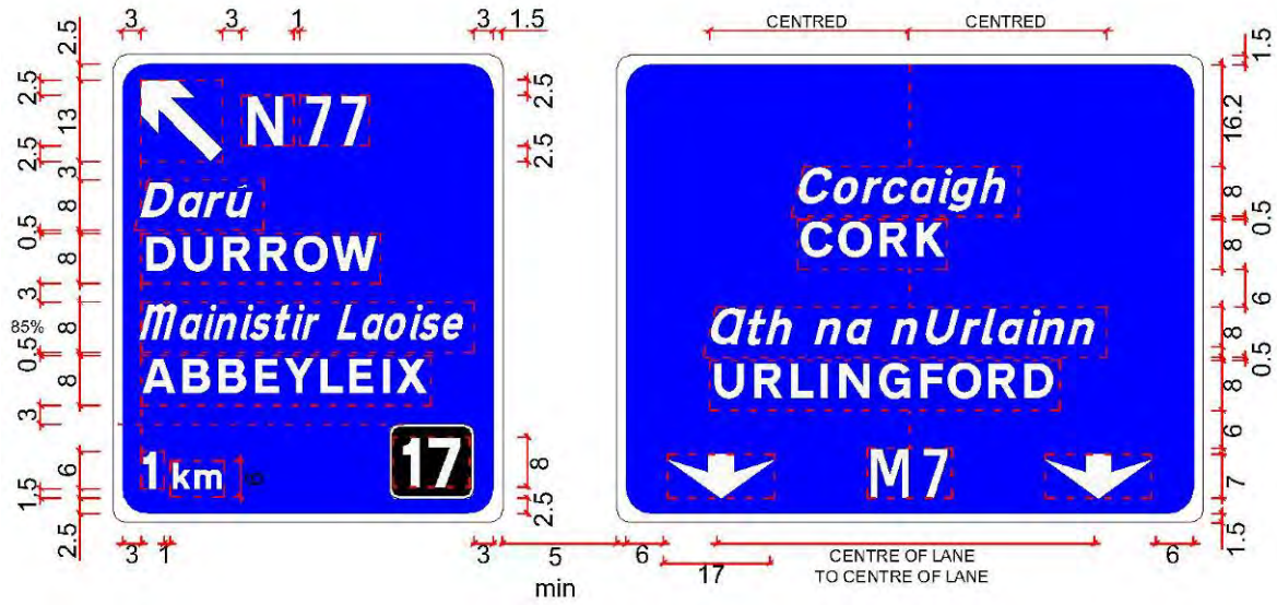
Figure 2.4.17: 1km Non-Lane Drop Gantry Sign
