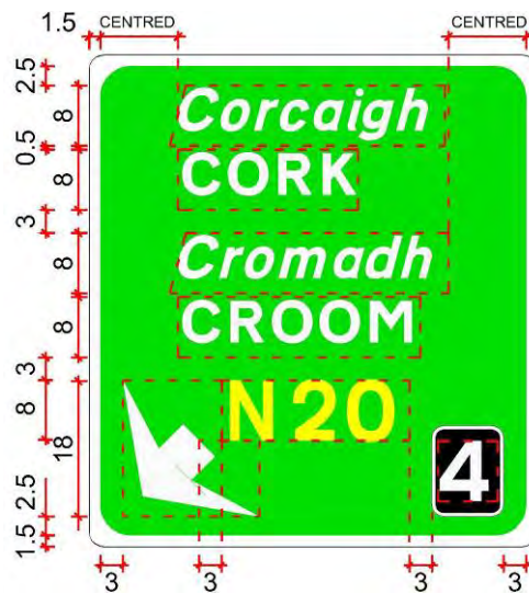
Figure 2.5.20: National Route Exit Taper Gantry Sign
