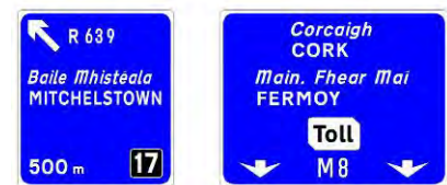
Figure 2.4.16: Non-Lane Drop Gantry with Toll Symbol.
