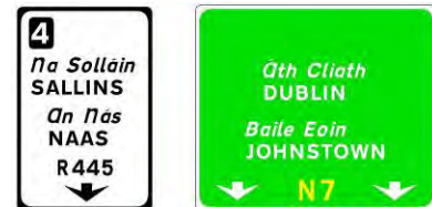
Figure 2.5.14: Typical Lane Drop Gantry Sign at a Diverge
