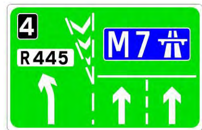
Figure 2.4.46: Lane Destination Sign at the Start of a Motorway.
