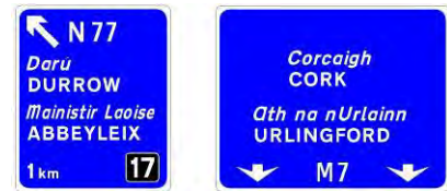
Figure 2.4.14: Non-Lane Drop Gantry at 1km
