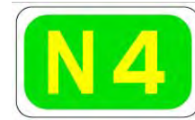
Figure 2.5.47: Typical Route Marker Sign for National Route
