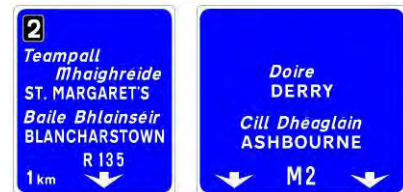
Figure 2.4.12: Typical Lane Drop Gantry
