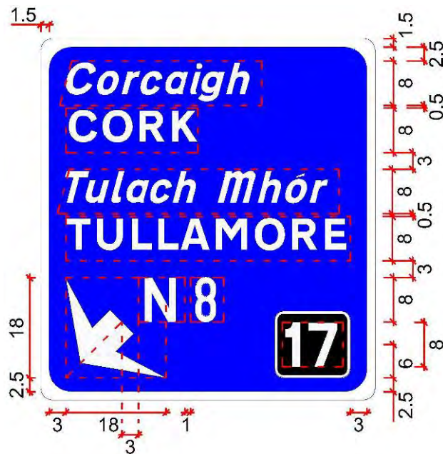
Figure 2.4.29: Exit Taper Gantry Sign for a National Route
