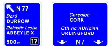
Figure 2.4.15: Non-Lane Drop Gantry at 500m
