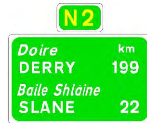
Figure 2.5.37: Typical Route Confirmatory Sign.
