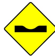
W 131: Road Depression
