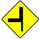
W 018L Junction With Major Road at Sharp Corner - Left
