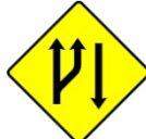
W 103 Start of Climbing Lane
