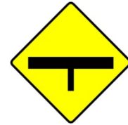
W 016: T-junction (Major Road) Ahead
