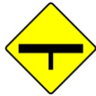
W 016 T Junction (Major Road Ahead)
