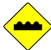
W 133: Uneven Road
