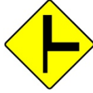
W 018R Junction With Major Road at Sharp Corner - Right
