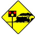
W 120 Level Crossing With Flashing Red Signals
