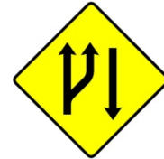
W 103: Start of Climbing Lane
