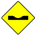
W 131 Road Depression
