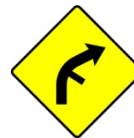
W 010R Side Road on Inside of Right Bend
