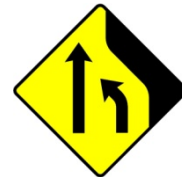
W 091R: Lane Loss (Two to One Lane)
