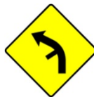
W 010L Side Road on Inside of Left Bend
