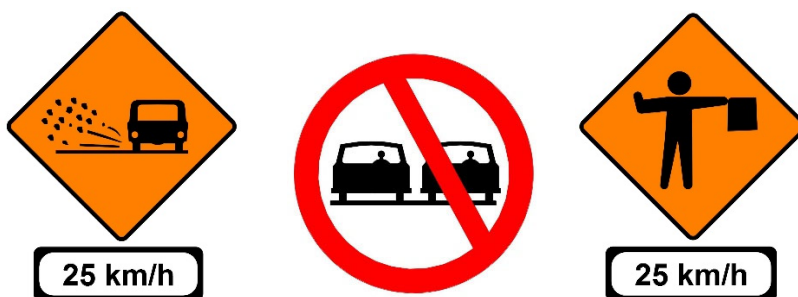
Figure 2.2.2.4: SSO Repeater Signs
