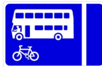
RUS 028 Nearside With-Flow Bus Lane
