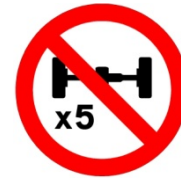
RUS 046: PROHIBITED NUMBER OF AXLES (For Goods and Other Non- Passenger Vehicles)
